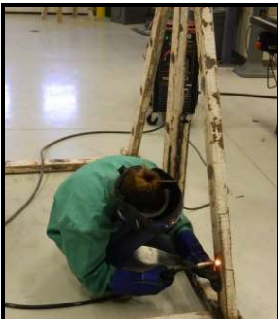
Tracey Long welds a training station for the Elida H.S. Track Team. Members cut, prepped and wire brushed the recycled tubing before welding.
